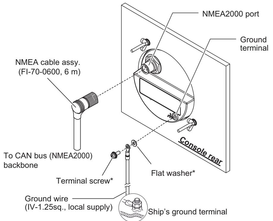
\*: Attached to FI-70 when shipped. Remove the terminal screw and washer to install.
