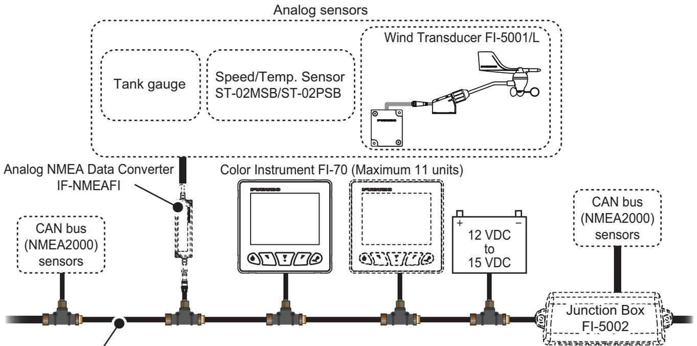
CAN bus (NMEA2000) Backbone: Terminal resistors must be installed at both ends of the backbone.
