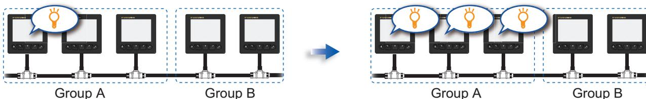
Grouping the FI-70 units eliminates the need to adjust each unit individually. Up to three groups (A, B, C) may be set up.
